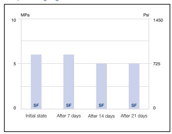
¹ Immersion in water | ² Thermal cycling 100 cycles (2h at -30°C / 1h up to 70°C / 2h at 70°C / 1h down to -30°C) | SF: Substrate failure
