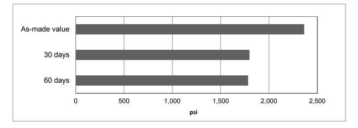
Lap shear strength versus immersion in various media (ASTM D1002) (typical average values). Cured 7 days at RT Tested at 23°C (73°F). Lap Shear Strength was determined after immersion for 30, 60 and 90 days at 23°C (73°F).
