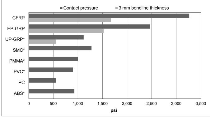
(\*): UP-GRP, SMC; PMMA, PVC, substrate failure observed.
