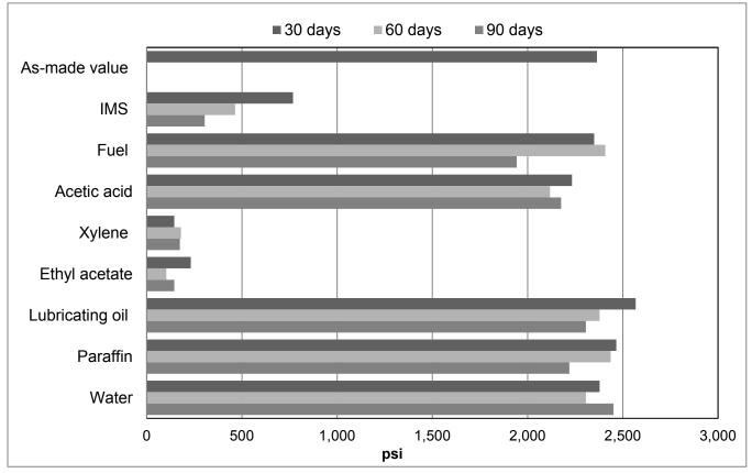
Lap shear strength (ASTM D1002) versus Cataplasma ageing (typical average values). Cure 24 hours at  $23^{\circ}C$  ( $73^{\circ}F$ ) – per ISO 9142/E2. Tested at  $23^{\circ}C$  ( $73^{\circ}F$ ). Metals: sandblasted and degreased; Plastics: abraded and degreased.
