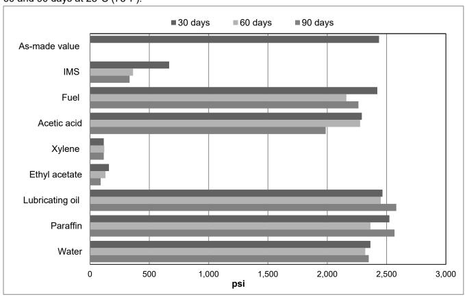
**Lap shear strength (ASTM D1002) versus Cataplasma ageing** (typical average values). Cure 24 hours at 23°C (73°F) – per ISO 9142/E2. Tested at 23°C (73°F). Metals: sandblasted and degreased; Plastics: abraded and degreased.
