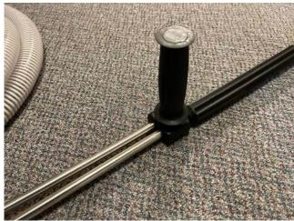
Twist handle to redirect water flow between upper and lower lances. This allows for variable pump speeds and extra water for tank mixing.
