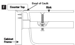
Start Adjusting Bolts into nuts and slide into position in rails and attach plastic caps (B). They should be evenly located along the underside of the sink deck.
