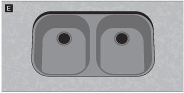
With the countertop now in place check to see that the sink is centered properly in relation to the cut out of the countertop. Raise the sink up by tightening the adjusting bolts until there is a watertight seal between the countertop and the sink deck. Remove excess caulk.
