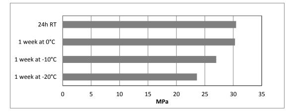
Average lap shear strengths after application, bonding and curing under water (ISO 4587) (typical average values)
