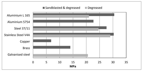
Notes: Araldite<sup>®</sup> 2050 is not suitable to bond copper or brass without surface preparation. Galvanised steel should not be abraded or sandblasted, better results are obtained with only degreasing.
