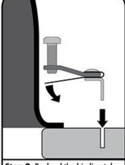
Step 2: Pre-load the binding tab by bending it away from the Slot-Klip body and fully insert the anchor post into the hole.
