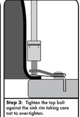
Please note: The countertop is shown upside down in these installation directions, but sinks can be mounted from underneath as well.
