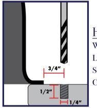
Hole specifications: Using a 1/4" bit on a drill with a minimum speed of 3000 RPMs, bore at least a 1/2" deep hole 3/4" from the edge of the sink rim. May bore hole up to 3/4" deep on 3cm countertops.
