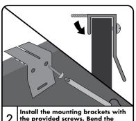
mounting tabs down over the cabinet divider for added strength.
