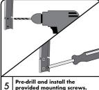
Pre-drill and install the provided mounting screws.
