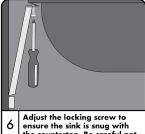
Adjust the locking screw to ensure the sink is snug with the countertop. Be careful not to lift the countertop.
