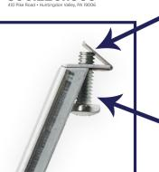
BINDING TAB: PREVENTS THE BOLT FROM "WALKING" ON THE SINK RIM. AS THE WEIGHT OF THE SINK PRESSES DOWNWARD, IT ALSO CREATES PRESSURE AGAINST THE BOLT, "LOCKING" IT IN PLACE.
