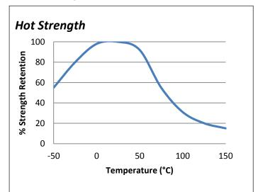
"Hot strength" shear strength tests performed on mild steel. 24hr cure at room temperature and conditioned to pull temperature for 30 minutes
