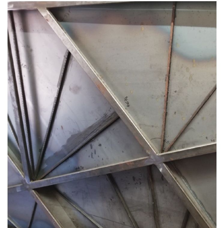
Metal Reinforcements onto an outer panel
