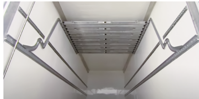
Logistic track bonded with Plexus adhesive
