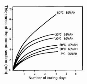
Relationship between curing speed and temperature/humidity
