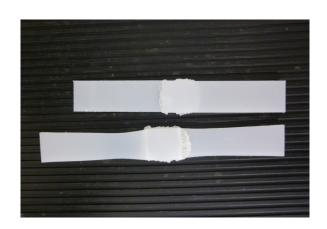
Polypropylene lapshears bonded with TA4610 . The adhesive bond is so strong the plastic stretches, deforms, and fails before the bonded joint.
