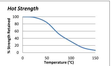
"Hot strength" shear strength tests performed on mild steel. Fully cured specimens conditioned to pull temperature for 30 minutes before testing at temperature. TA4207 can withstand higher temperatures for brief periods (such as for paint baking and wave soldering processes) providing the joint is not unduly stressed. The minimum temperature the cured adhesive can be exposed to is -40°C (-40°F) depending on the materials being bonded.
