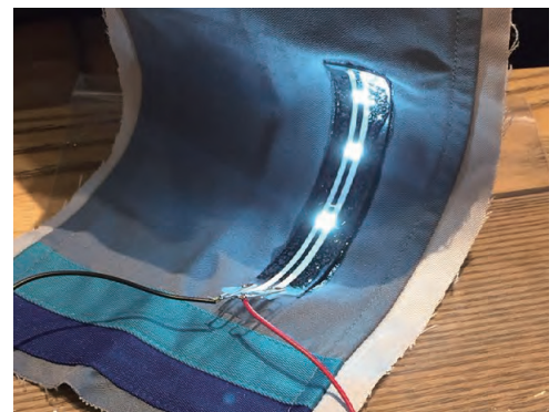
LED is lit by conductive silicone rubber circuit on the cloth.
